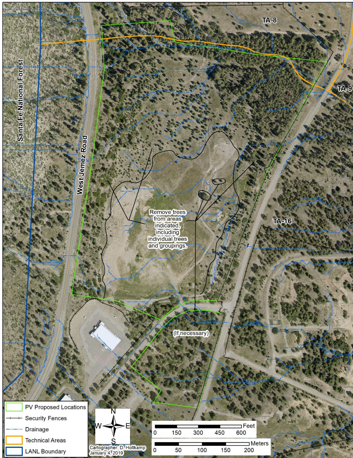
Figure 2-8: PV Array Site Preparation Potential Tree and Shrub Grubbing Areas.
