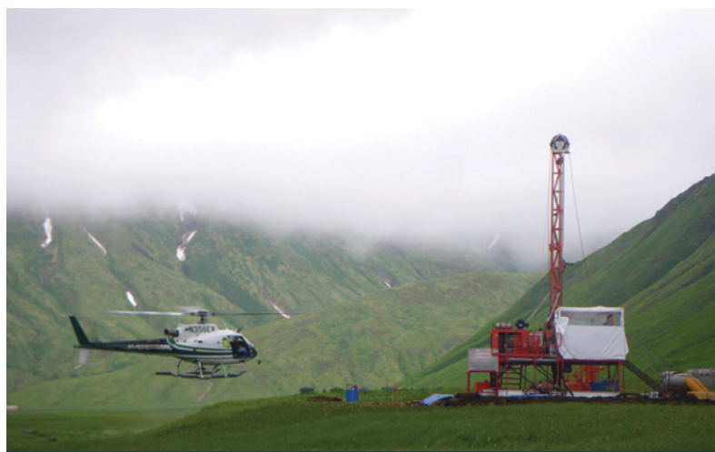
Helicopter-supported geothermal exploration drilling on Akutan Island, Alaska. Photo credit: Neil McMahon
