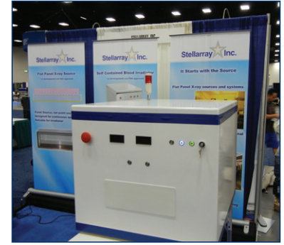
A complete, operational prototype blood irradiator using Stellarray's novel flat panel X-ray sources.
