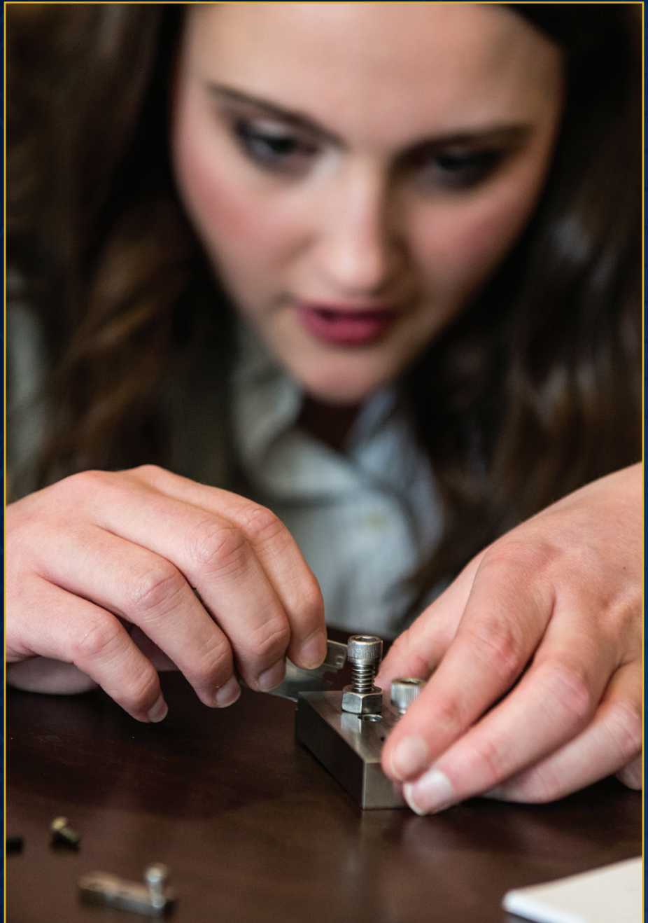
Washington State University student Jacqueline Reeve assembles an apparatus that bends the metal filament to hold samples for thermal ionization mass spectrometer analysis. NNSA's Office of International Nuclear Safeguards Human Capital Development program brings together PNNL safeguards researchers and WSU students enrolled in WSU's Industrial Design Clinic. Photo credit: Maren Disney | Pacific Northwest National Laboratory
