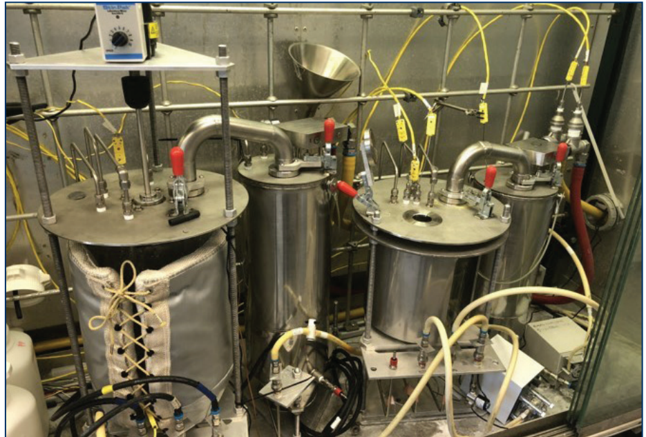
Argonne National Laboratory designed and built a full-scale dissolver to dissolve irradiated molybdenum targets. (Photos courtesy of M3)
