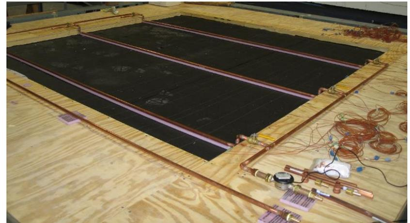
Prototype TAC wall being built for large-scale test
