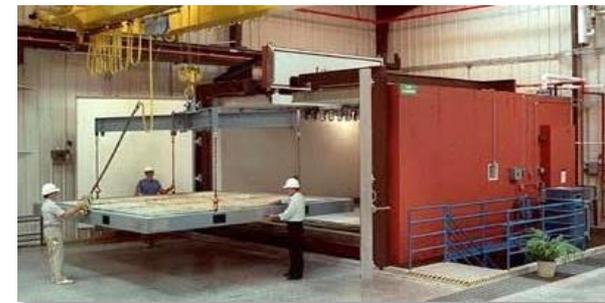
Large-scale climate simulator for prototype tests
