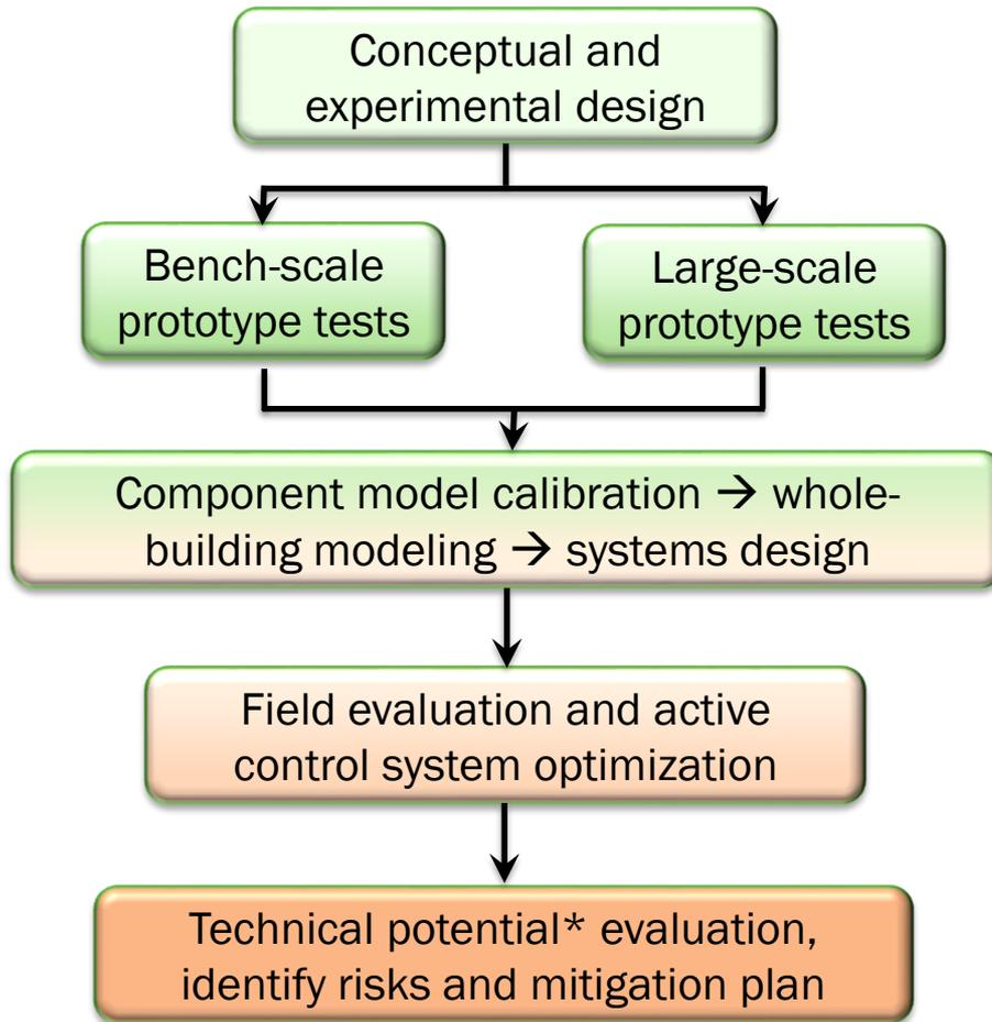
\*Energy savings, peak load reduction, and thermal energy harvesting potential under various weather conditions using field data and simulations.
