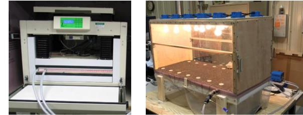
Heat flow meter apparatus and custom-built setup for proof-of-concept and bench-scale tests
