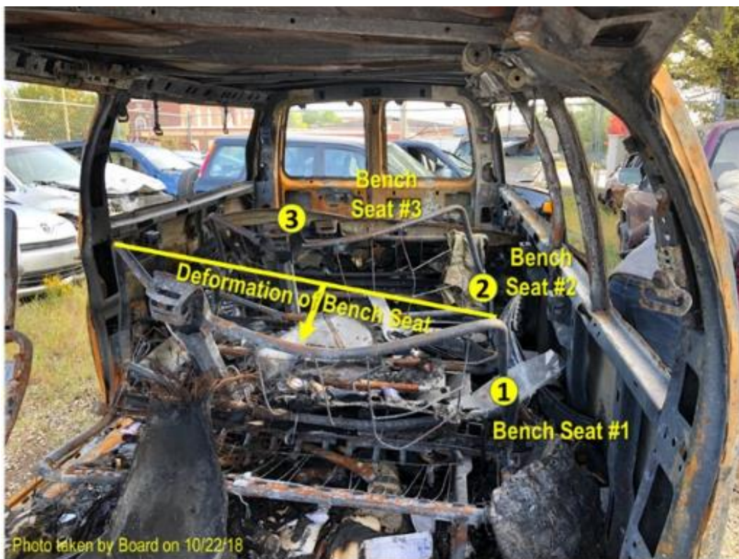
Figure 2-22. Deformation of Bench Seats by Occupant Impact (Frontal View)
