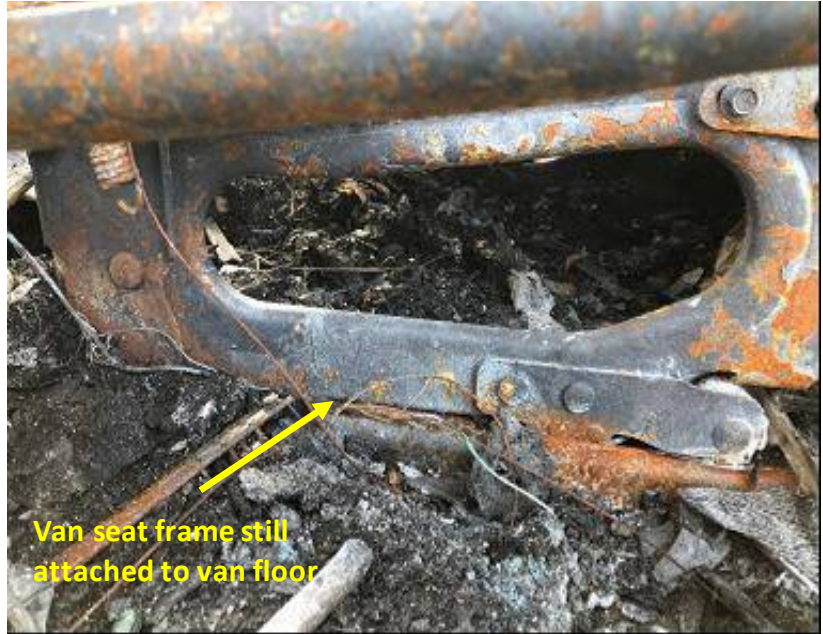
Figure 2-8. Bottom Frame of Van Seat
