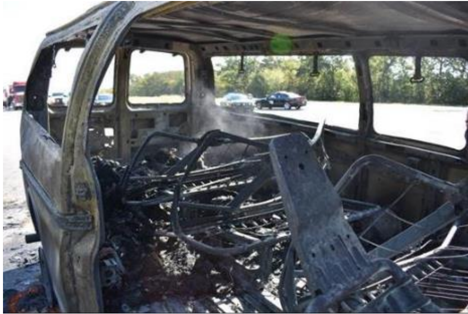
Figure 2-10. Inside View of Van Damage from Fire and Collision
