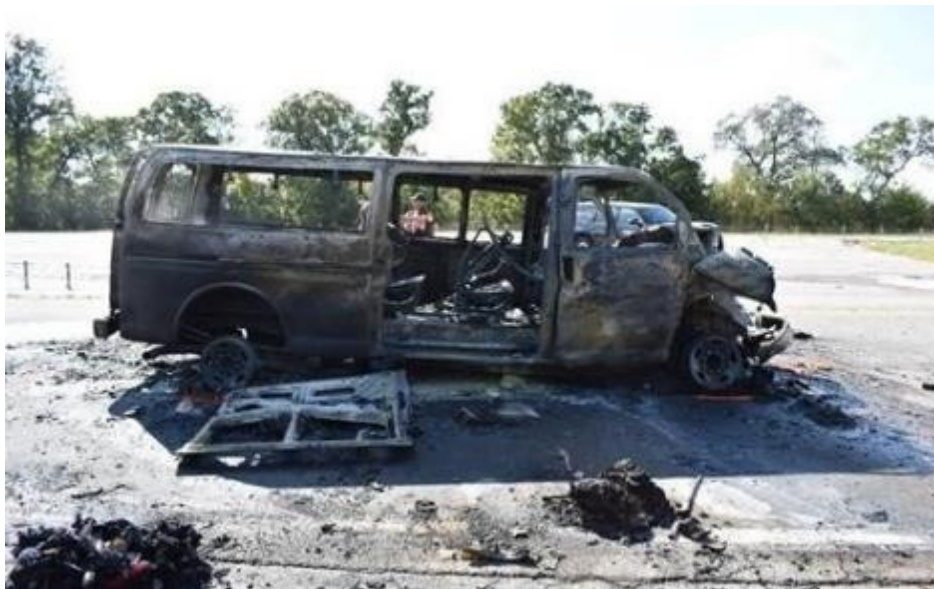
Figure 2-9. Side View of Van Damage from Fire and Collision
