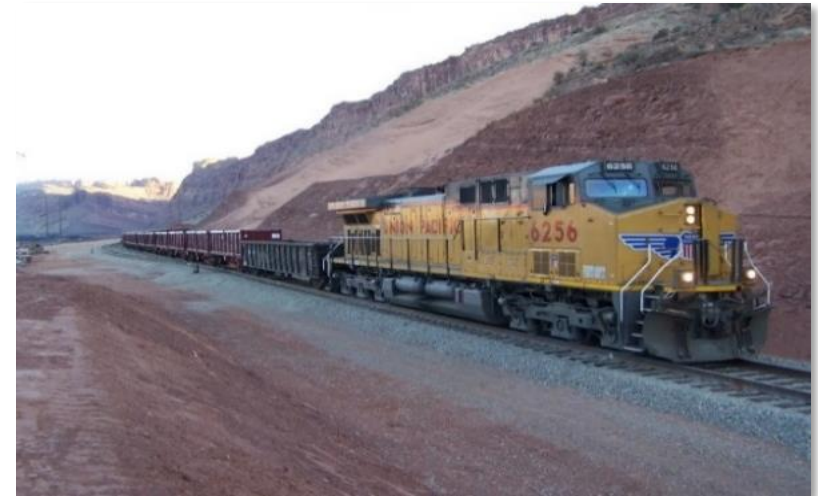
Locomotive transports sealed containers of tailings from Moab to a disposal site
