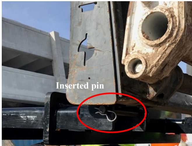
Figure 6: JLG Forklift Attachment on Bobcat with Safety Pins Installed.
