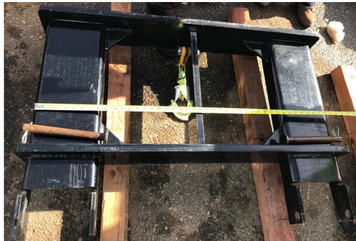
Figure 4: JLG Telehandler Forklift Attachment with Safety Pins Not Inserted.
