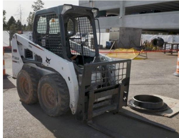
Figure 5: Bobcat S450 Skid Steer Loader used on day of the accident.
