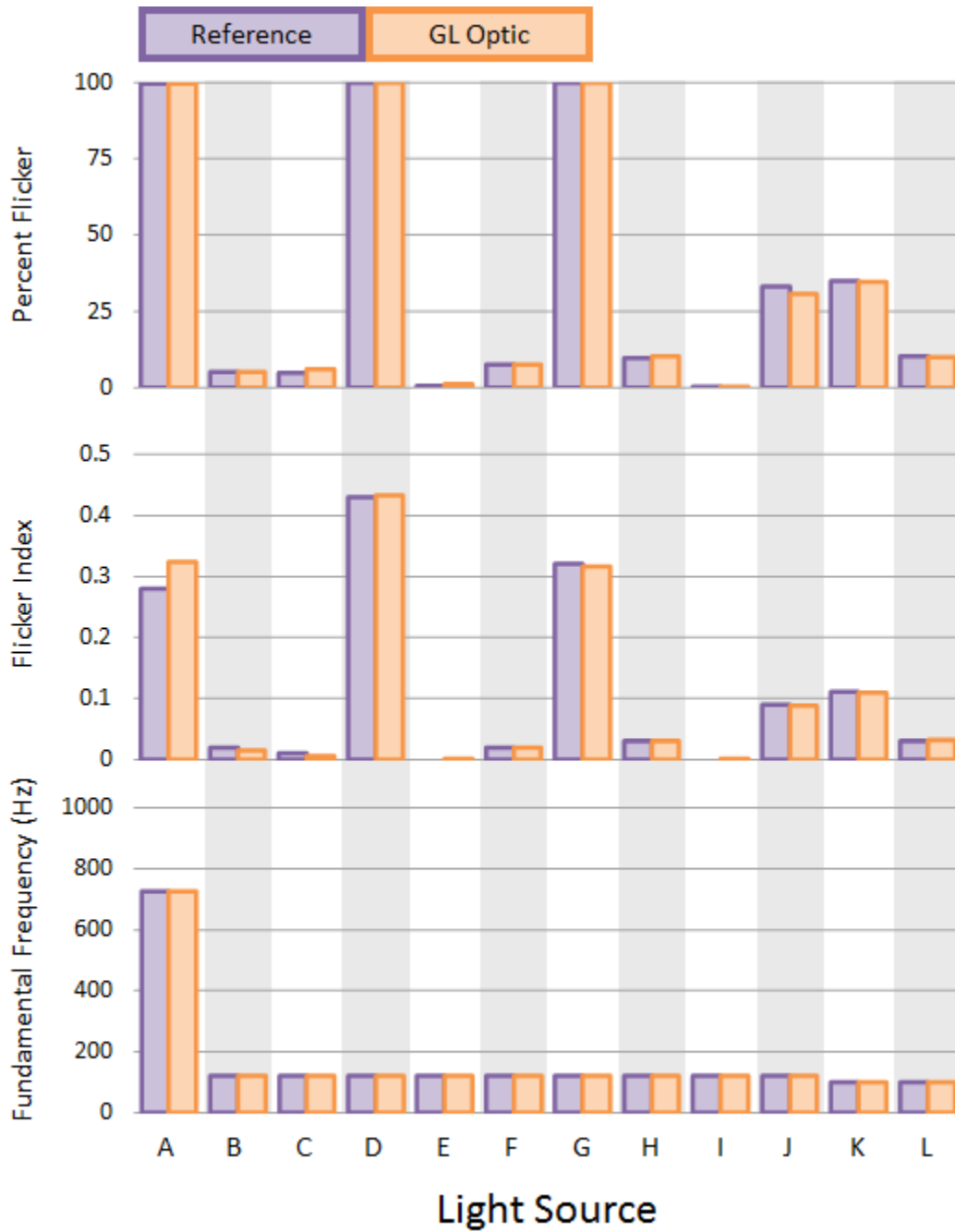
Figure 19. GL Optic and reference meter flicker metrics for the various light sources tested.
