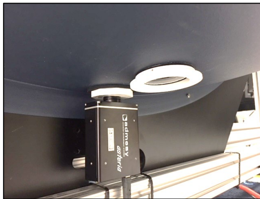
Figure 2. Positioning of reference and handheld flicker meters on integrating sphere.
