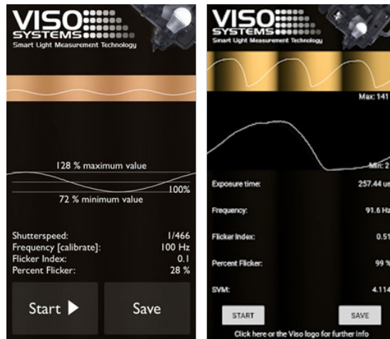
Figure 4. Screenshots showing the Apple iOS (left) and Google Play Android (right) versions of the Viso Flicker Tester App.
