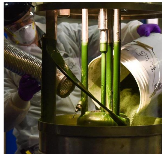
Skid 1 Hockmeyer Wet Mill
