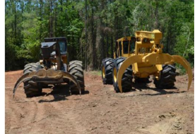
Enlarged grapple arms for the Tigercat wheeled skidder design developed through the DOE-funded Auburn University High-Tonnage Logistics Project
