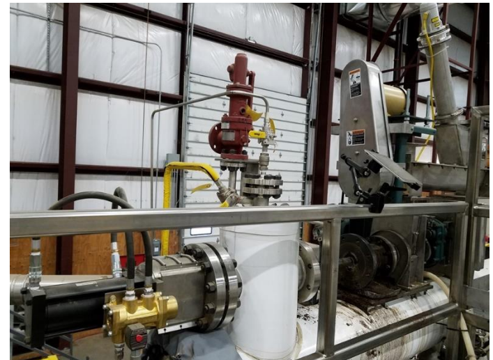
4" Plug Screw Feeder in INL's Biomass Feedstock Process Development Unit
