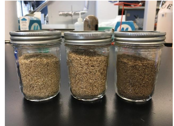
Corn stover without storage and treated with P. chrysosporium for 1 and 2 weeks (left to right)
