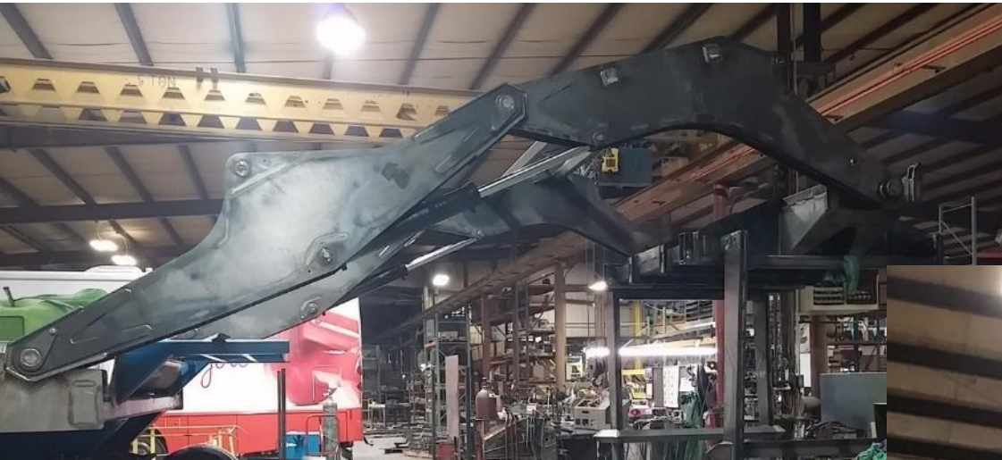
Loader arms and mast fabrication
