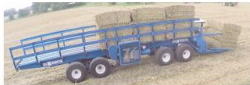
Bale Picking Truck; picks up to 6 bales at a time; 36 bales per trip
