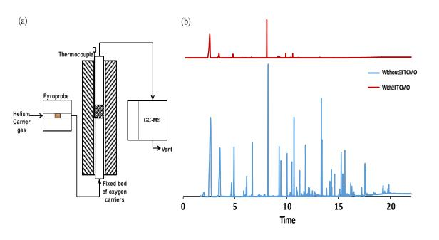
ITCMO oxygen carrier able to crack tar constituents in biomass
