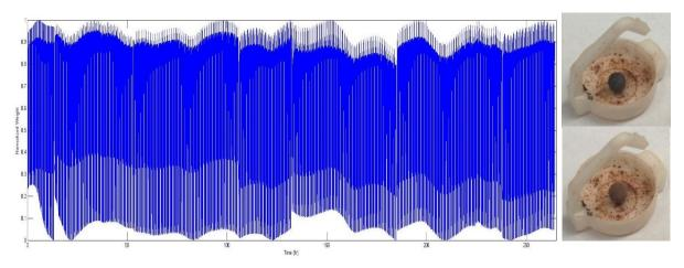
>1,000 redox cycles completed without loss in reactivity, recyclability, or strength
