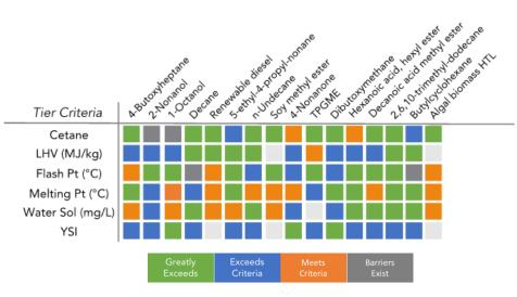
Boosted spark ignition (BSI) merit function and mixing-controlled compression ignition (MCCI) merit table approach to rapidly identify most promising candidates to meet targets.
