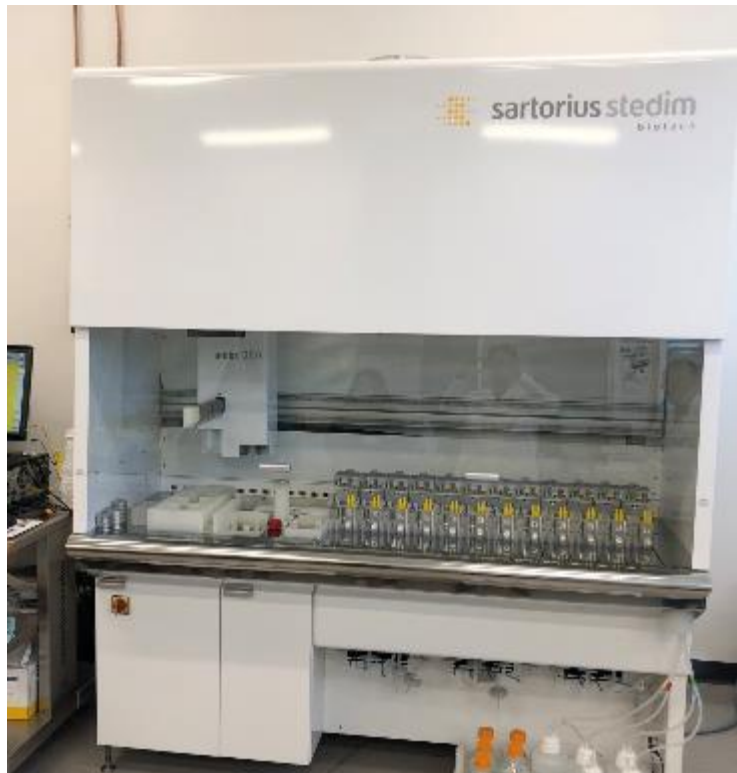
Ambr250 HT automated bioprocess dev't system
