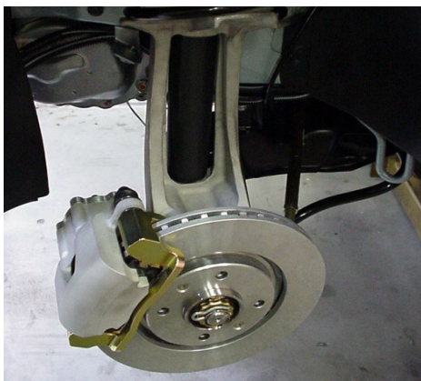
Figure 1. Example of lightweight aluminum corner unit. (Picture courtesy of Delphi Automotive.)
