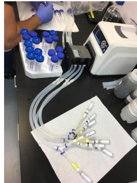
Filter through 0.22 \mu m Sterivex filter
