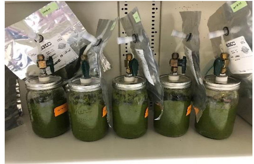
Anaerobic storage of S. acutus in 1-L reactors
