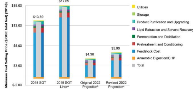
Figure 2-17: Cost contribution by process area for CAP Pathway
