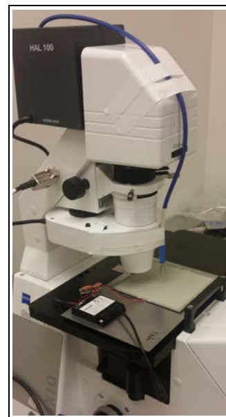
Figure 2-2. Testing configuration for luminance measurements.
