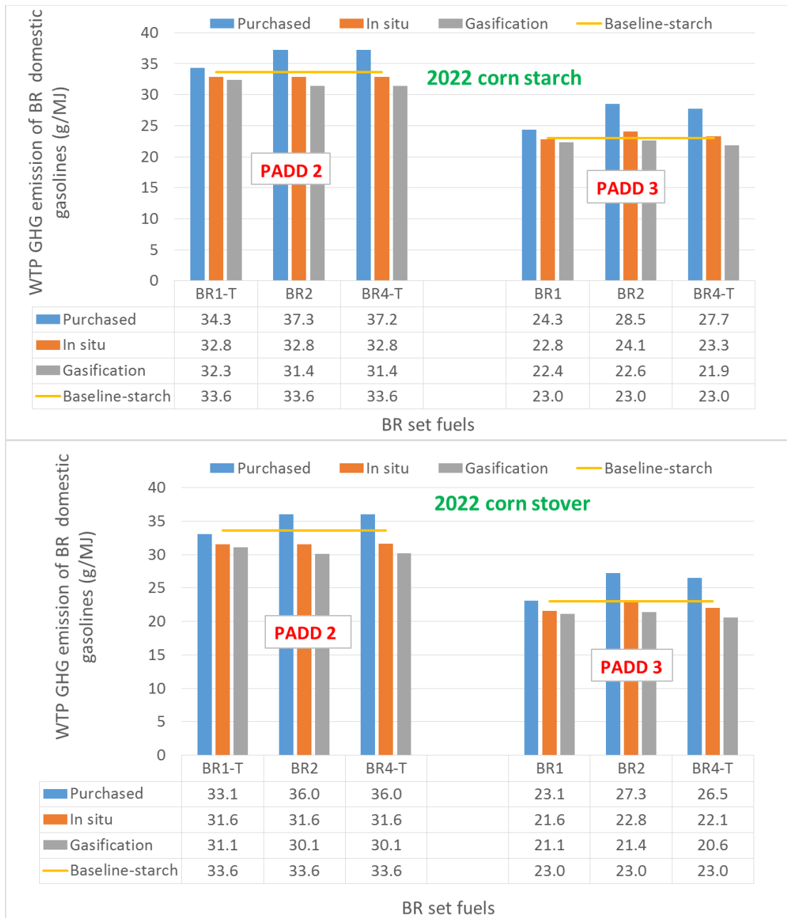
Figure A3-16. WTP GHG Emissions of BR Set Domestic Gasolines Produced in PADD 2 and PADD 3 refinery in 2022 (g/MJ Domestic Gasoline). Baselines Use Corn Starch Ethanol.
