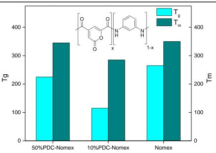
Consistent thermal properties with Nomex, lower T<sub>g</sub> leads to easier processing
