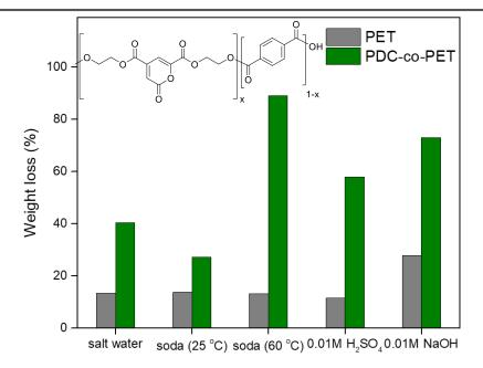
Lower resistance of PET-PDC enables facile recycling at same properties
