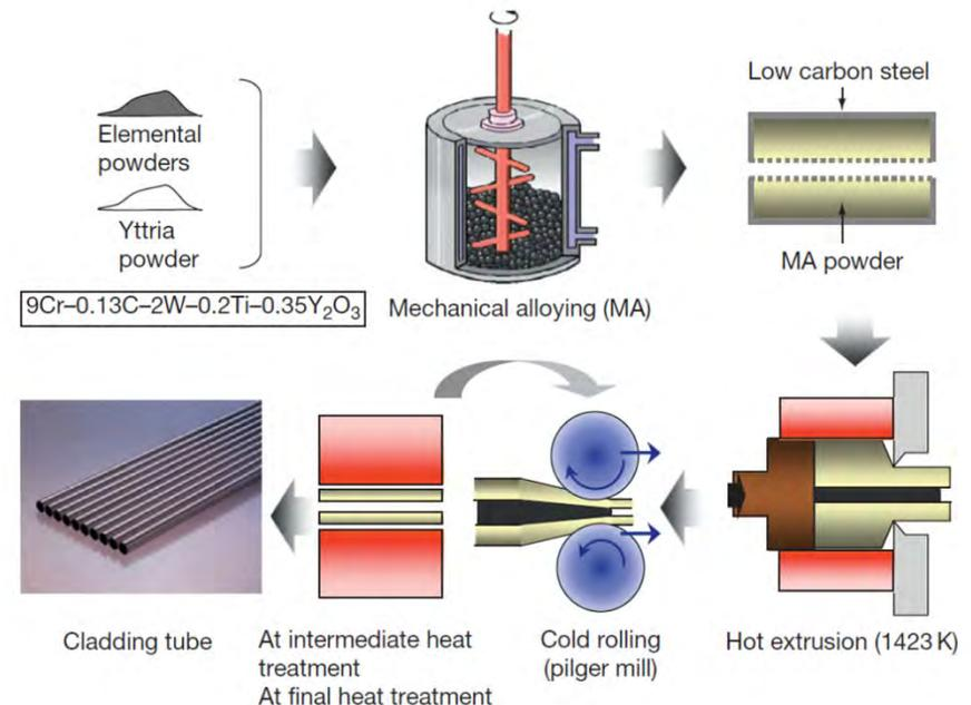
**Conventional fabrication of ODS steel tubes requires multiple extrusion steps [3]**
