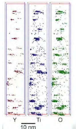
TEM image showing nano-scale oxide particles in ferritic matrix of ODS steel [1, left] and atomic probe tomography (APT) image of nanoparticles [2]
