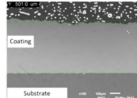
**Zn cold spray coating on steel substrate**
