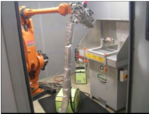
**Robot for pre-programmed movement of spray gun**
