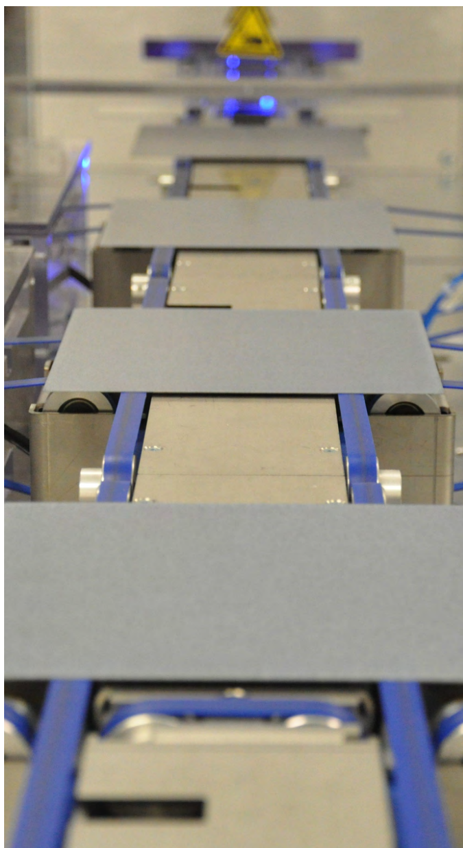
Silicon solar wafers move down a conveyor belt following a quality check.
