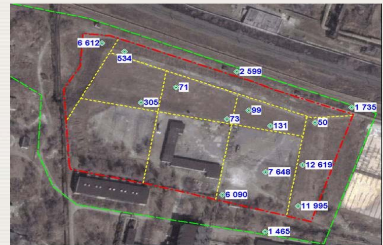
Distribution of Rn-222 flux (mBq/m 2 /s) from the surface of Zapadnoe tailings in September 2009
