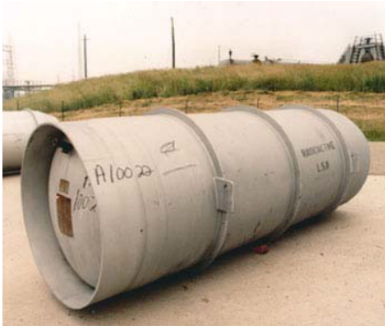
Figure S-3 Typical Depleted Uranium Hexafluoride Storage Cylinder (Source: ANL 2001)
