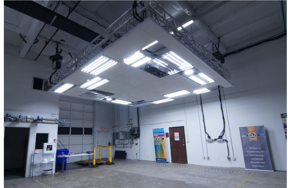
Luminaires spaced 14' o.c., mounted 11'-3" above floor
