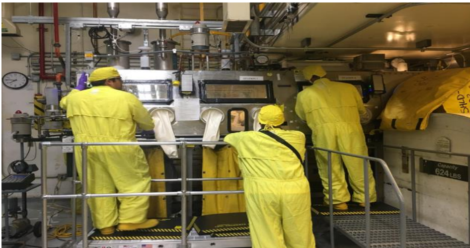
Technicians at the glove box inside WCRRF
