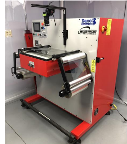
R2R film inspection station with Automated Dynamics machine vision system commissioned February 28
