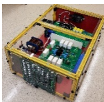
25 kVA 5 kV Dc to 600 V DC Building Block Based on 3.3 kV SiC current Switch
