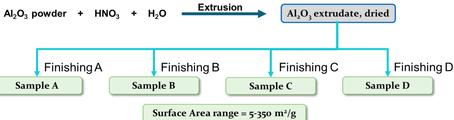
For each sample A through D, platinum loading via impregnation at two levels:
