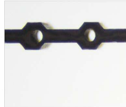
Fintube Prototypes for Proposed GCMC HX (TRL3 Demo)
