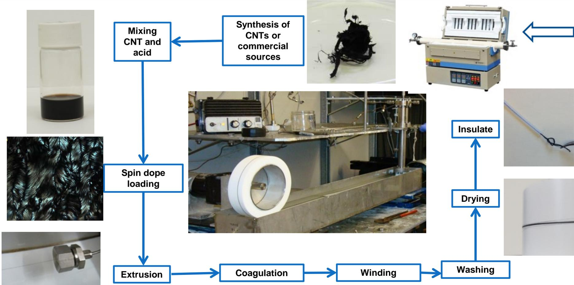
**Our approach:** scalable & allows independent optimization of CNT synthesis & fiber spinning
