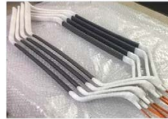
Prototype Litz coils
