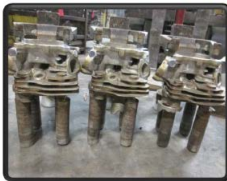
Cast Al-Ce Engine Head Before Machining
