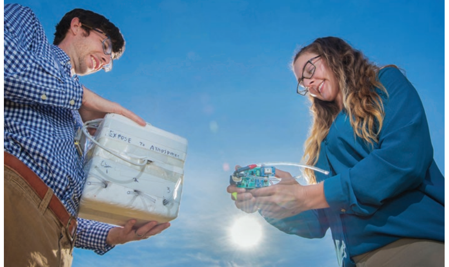
Sandia National Laboratories geophysicists Danny Bowman and Sarah Albert display an infrasound sensor and the box used to protect the sensors from the extreme temperatures experienced by balloons that take the sensors twice as high as commercial jets fly. Photo by Randy Montoya, Sandia National Laboratories.
