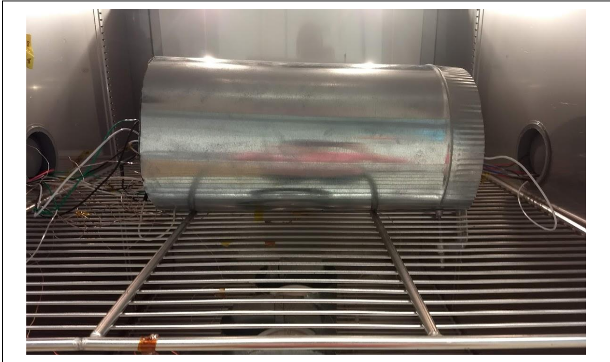
Figure 4-1. A metal dome was added around the DUTs during AST exposure
