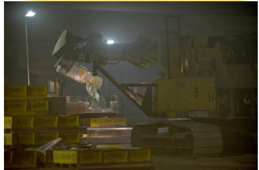
(Above) An excavator empties drum contents onto a sorting table as part of the treatment process.
