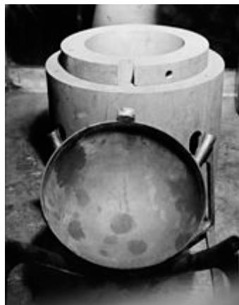
(Left) Graphite mold for plutonium pit production (right) machining lathe
