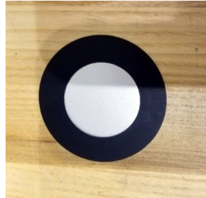
Figure 3. Sealed radioactive source
