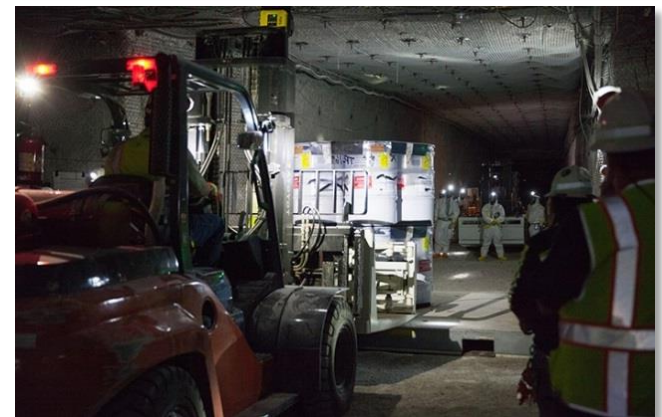
Waste Emplacement at the Waste Isolation Pilot Plant
