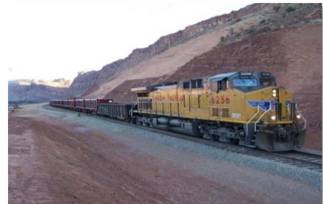
Locomotive transports sealed containers of tailings from Moab to a disposal site
