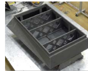
First building in the world with a façade made with 3D printed molds
