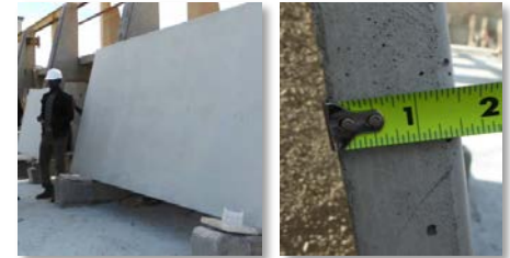
High-performance concrete mix for 1.5”-thick wythes
