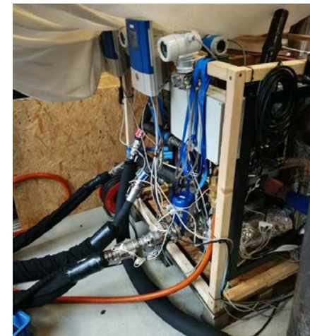
Vessels connected to the glycol loop and heating fluid loop at the testing facility
