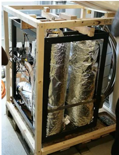
Vessels mounted on a skid with the burner, hybrid heat pipe, and controls
