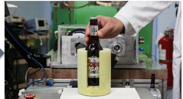
Demo Magnetic Refrigerator Source: GEA (2015)
