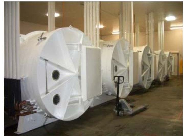
Example of an industrial facility equipped with dryers with a capacity of 1500 kg).
