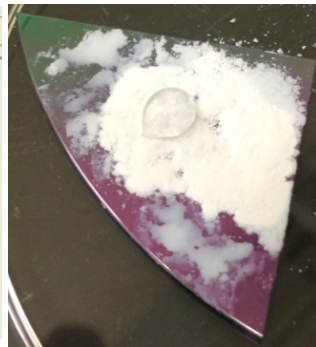
DDMS (Short Chain) treated (left) Si wafer with contact angle 95.5^{\circ} (right) pressed nanoparticle
