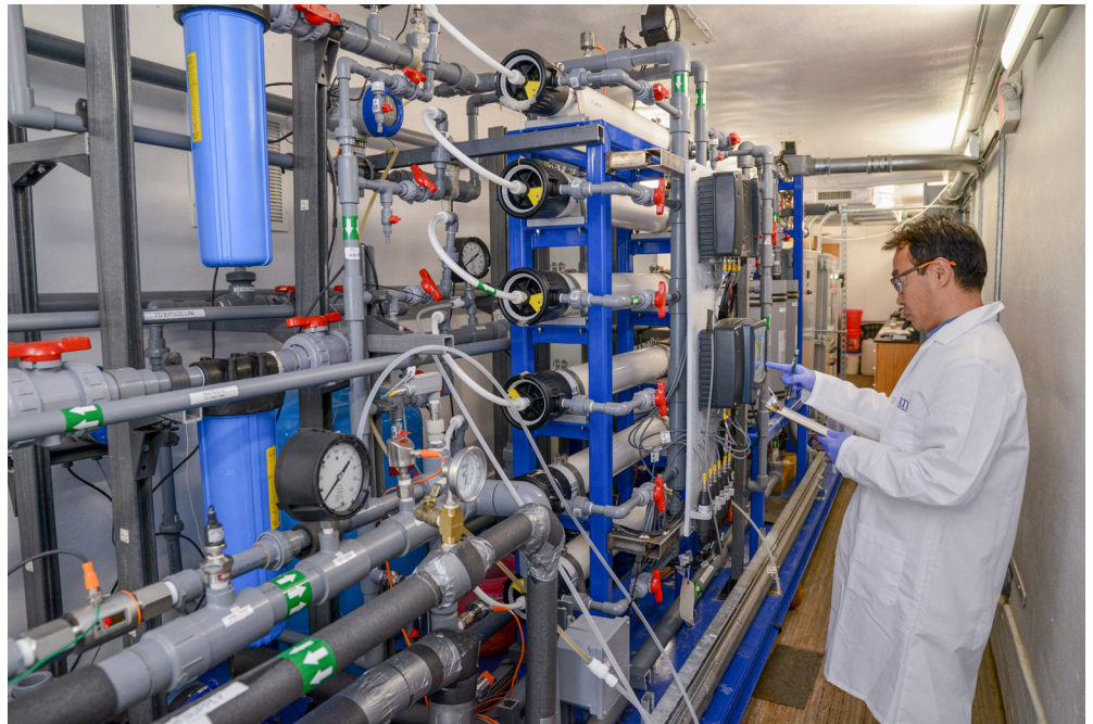
Pilot-scale hybrid FO/MD membrane system prototype in operation treating produced water. Photo credit RTI International.
