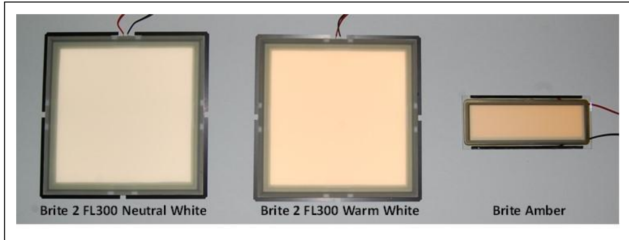
Figure 3-2. Neutral white, warm white, and amber panels from OLEDWorks.
