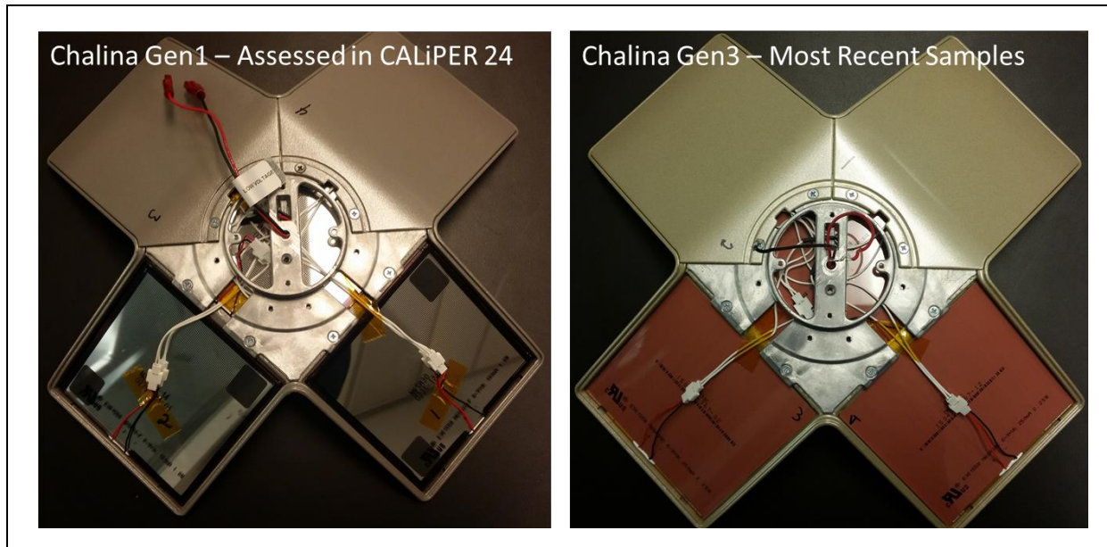
Figure 3-1. View of the backside of Chalina OLED luminaires from Acuity Brands.
