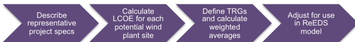
Figure H-9. Land-based wind plant cost and performance techno-economic parameter calculation process
