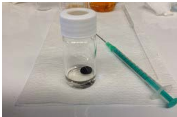
Figure II-613. Photograph of cathode discharged to 1000 mAh/g, dried under Ar for 1 hr, and then soaked in 3 mL of \text{TiOSO}_4(\text{aq}) . No apparent color change occurred upon titration indicating no \text{Li}_2\text{O}_2 is present
