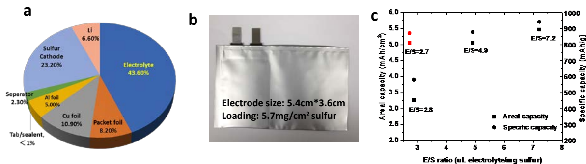
Figure II-563. (a) Component weight distribution of Li-S battery with energy density of 300 \text{ Wh kg}^{-1} , (b) photo of single-layer pouch cell used in present study (Electrode working area 19.4 \text{ cm}^2 and sulfur mass loading 5.7 \text{ mg cm}^{-2} ), and (c) dependence of first-discharge areal capacity and specific capacity on electrolyte/sulfur ratio (black symbol - pouch cell using pristine separator; red symbol - pouch cell using modified separator).
