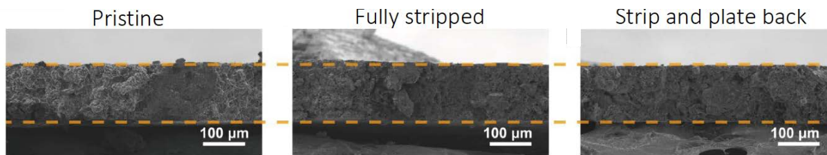
Figure II-626. SEM images of the cross section of a porous 3D host for Li metal plating and stripping, demonstrating its macroscopic dimensional stability.
