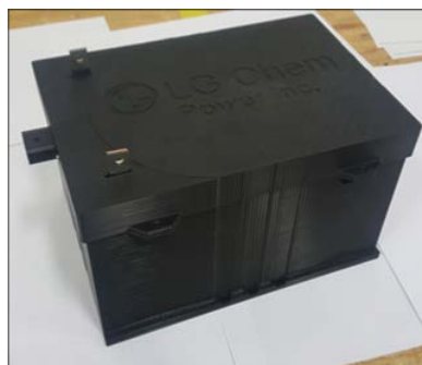
Figure I-31. Picture of the 12V Li-ion Start-Stop battery pack delivered to USABC for testing.
