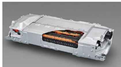
Figure I-69: 2016 Toyota Prius Lithium-Ion Battery Pack Specification Summary
