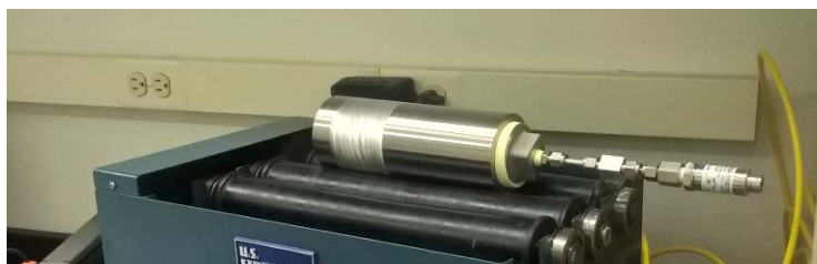
Figure II-25. Image of reactor vessel on roller mill. Note the pressure gauge pointing to the right.
