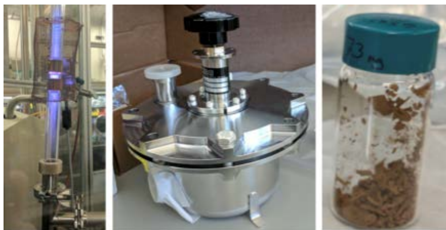
Figure II-145. Scaled-up plasma reactor, load-lock collection system, and small-diameter ( <10\text{-nm} ) hydrogen-passivated Si NPs.
