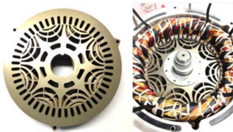
Figure 1. ORNL's synchronous reluctance prototype motor lamination (left) and motor assembly (right).
