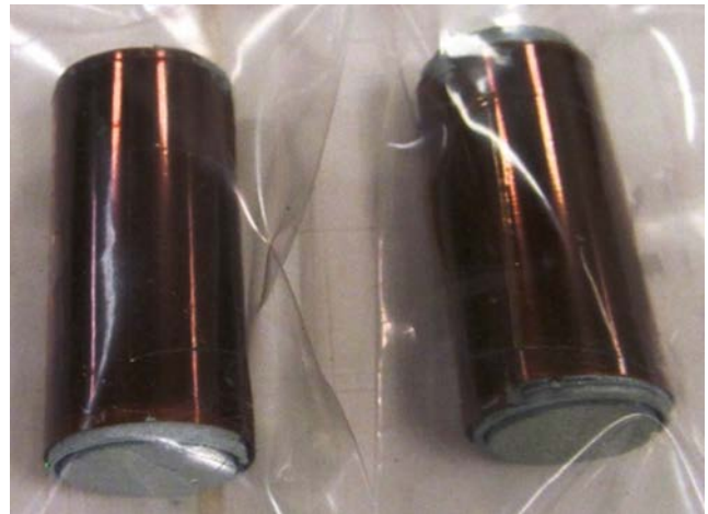
Figure 1. Long-length PLZT films were wound around a core with a separator layer of polyimide film, demonstrating the potential to make wound high-temperature ceramic capacitors.
