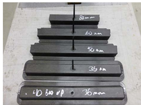
Figure 2. Mold fill profiles of the 3D complex part.
