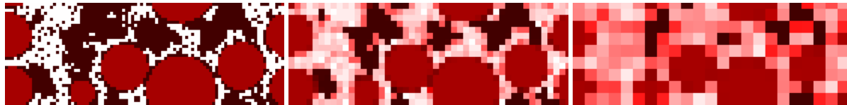
Figure V-198: Sequential coarse-graining procedure (left to right) used to speed up finite-volume conductivity calculation
