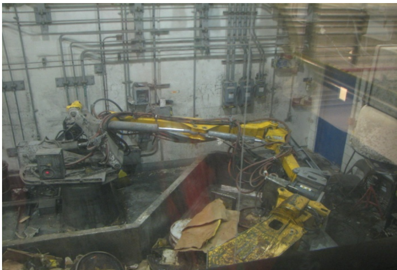
The North-West BROKK with a Broken #2 arm laying on it's side across the trough
